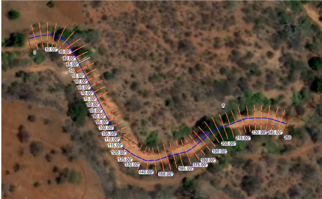
**Figure 4.18: Site 2 HEC-RAS reach geometry.** The HEC-RAS geometry for Site 2 shows the 53 cross-sections covering the reach, with the sand dam located at the 50 m river station.
