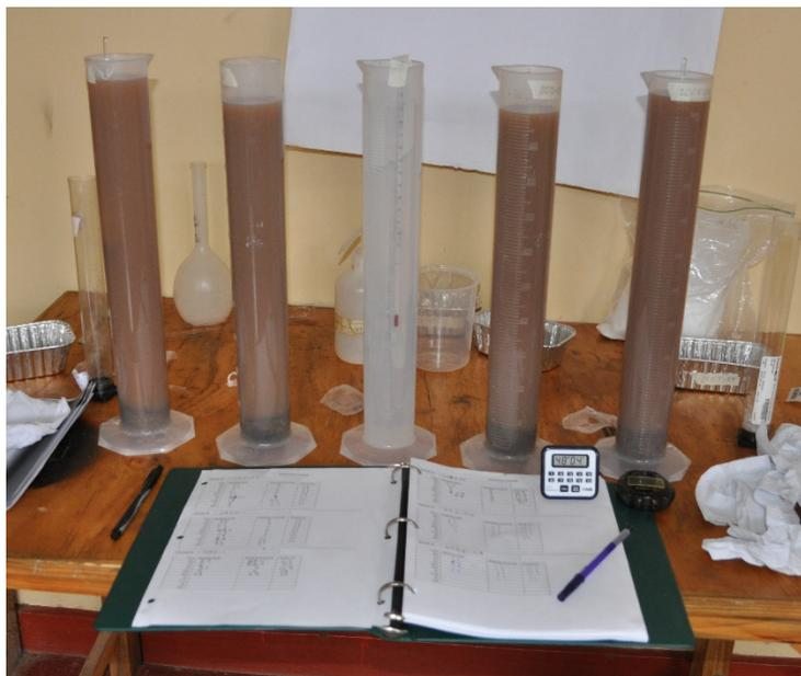
**Figure 4.6: Hydrometer test.** *Hydrometer tests were performed to measure the contribution of fine sediments to each sample's particle size distribution.*
