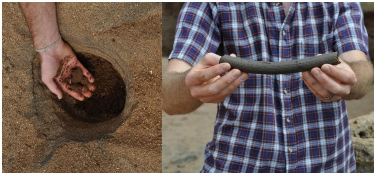
**Figure 4.7: Buried bottomset bed.** *Many sand dam storage volumes feature a thick bottomset bed of silt or clay, overlain by coarse sand.*
