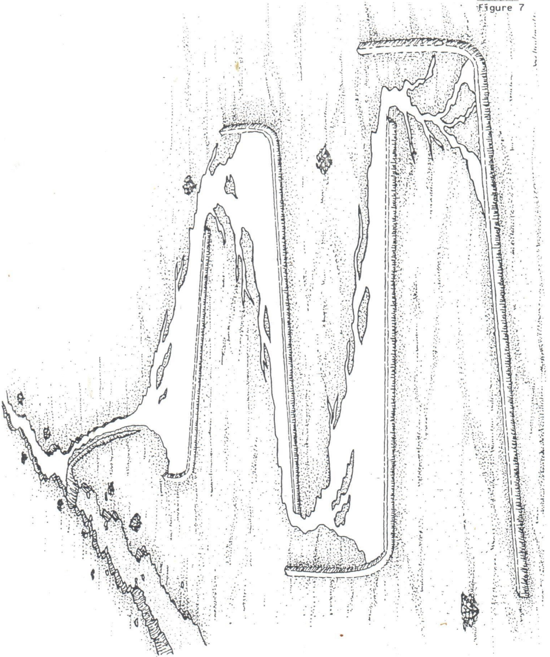
Flood diversion and water spreading for pasture and browse production. To and fro off-contour spreading bunds.
