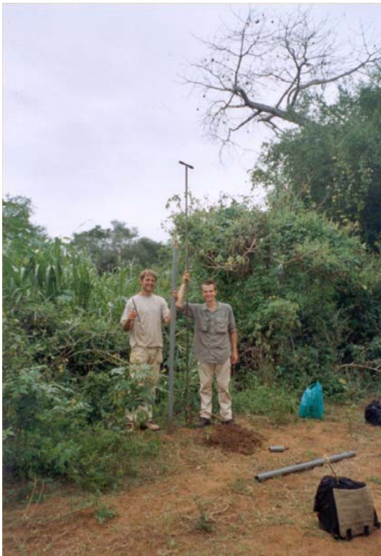
Figure 13: Auger next to a piezometer
