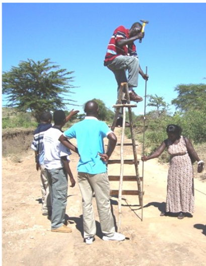
Photos: Probing with 6 m long iron rods.
