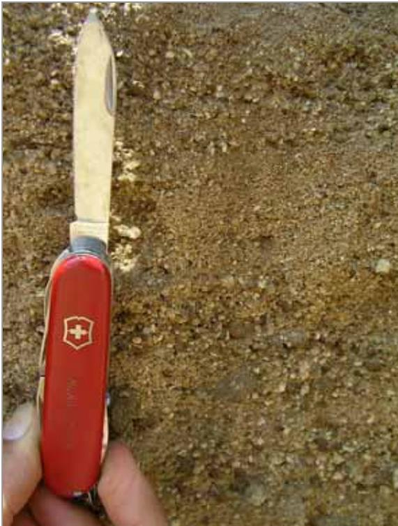
*Figure 2.13 The riverbed is filled with coarse sand*
