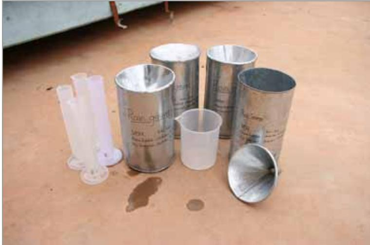
Figure 3.2 The locally produced totaliser rain gauges
