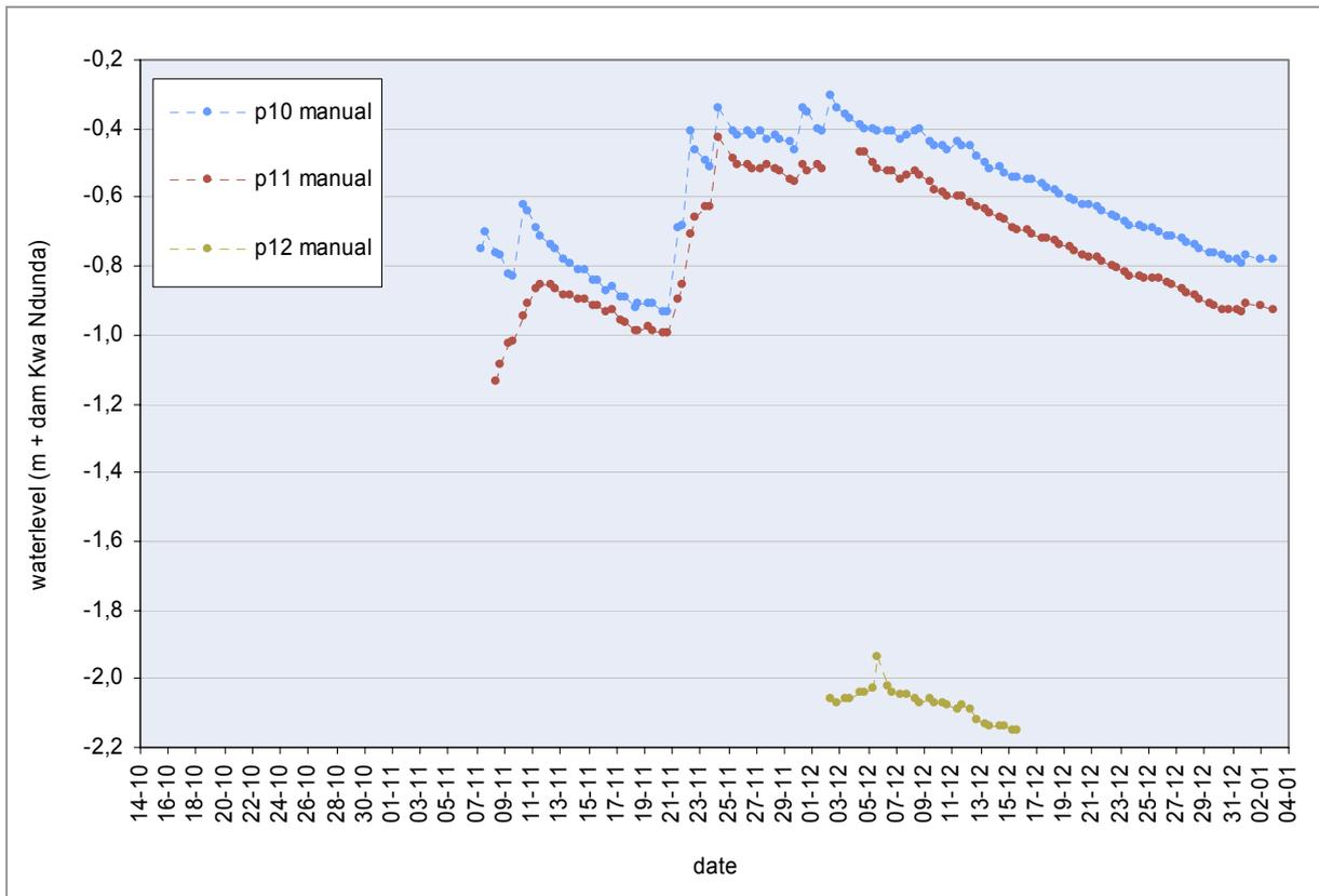
Piezometers next to dam Kwa Ndunda
