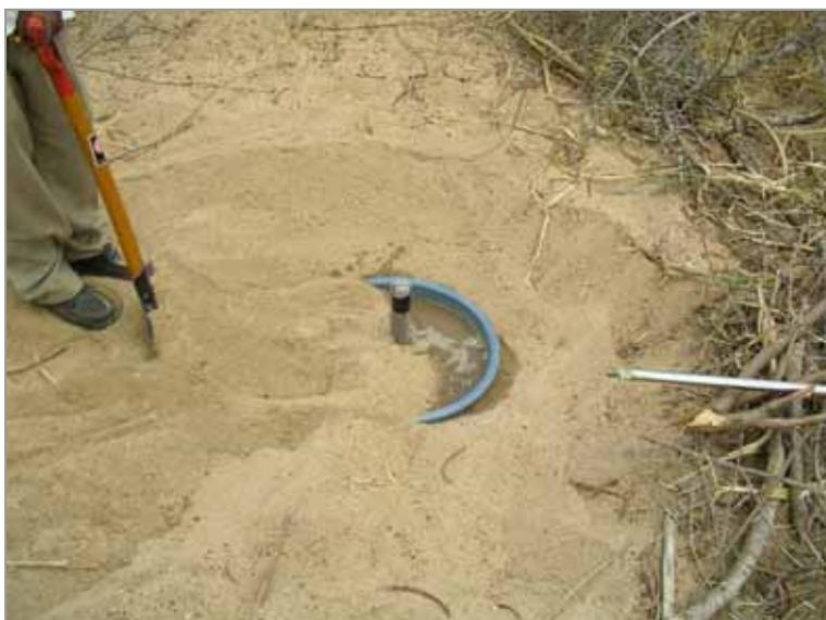
Figure 3.3 Sub-surface evaporation pan during installation
