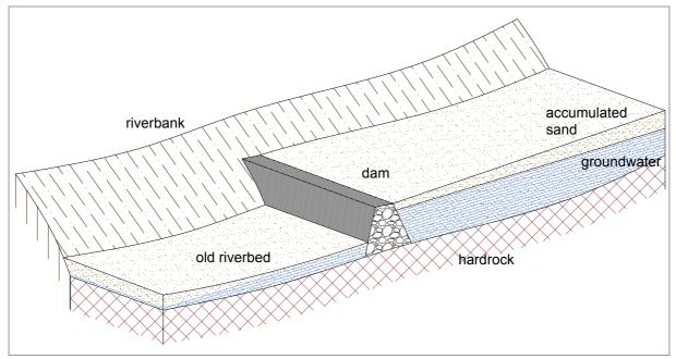
Figure 2.23 Principle of a sand storage dam
