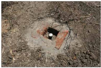
Figure 3.6 Piezometer
