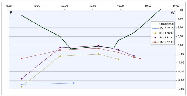
Figure 4.25 Upstream cross-section with changing water levels in time
