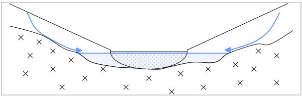
Figure 5.8 Schematic cross-section with lateral baseflow
