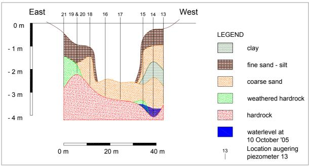
Figure 4.14 Downstream cross-section. The direction of sight is downstream
