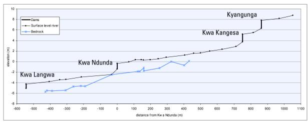
Figure 4.17 Longitudinal profile of the surface level of the river and the hardrock
