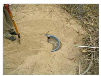
Figure 3.3 Sub-surface evaporation pan during installation
