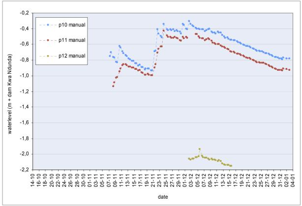
Piezometers next to dam Kwa Ndunda
