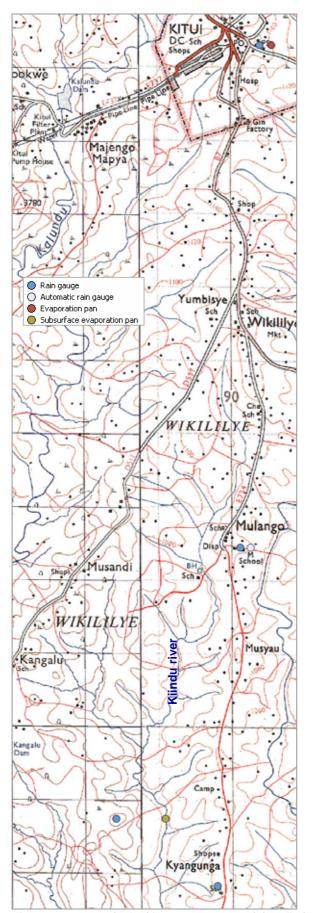
Figure 3.4 Meteorological instruments around the Kiindu catchment
