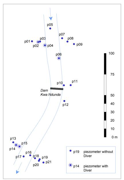
Figure 3.5 Overview of piezometers
