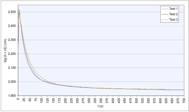
Figure 4.15 Results from inversed auger hole tests in piezometer 15
