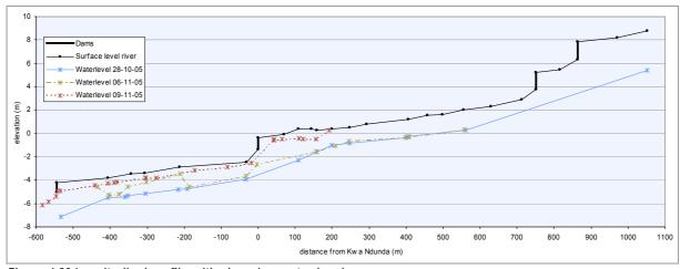
Figure 4.20 Longitudinal profile with changing water levels
