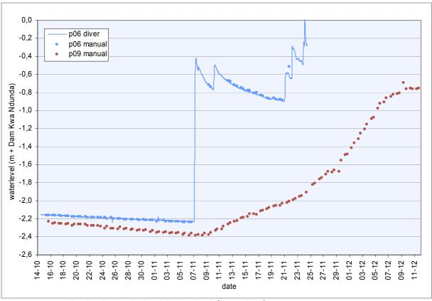
Figure 4.23 Water level in the riverbed and the riverbank (p06 and p09)
