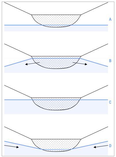
Figure 5.9 Schematic cross-sections over the riverbed: low water level (A), recharge from the riverbed to the banks (B), high water level (C) and recharge from the banks to the riverbed (D).
