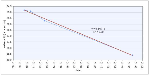
Figure 4.12 Observed evaporation in the sub-surface evaporation pan
