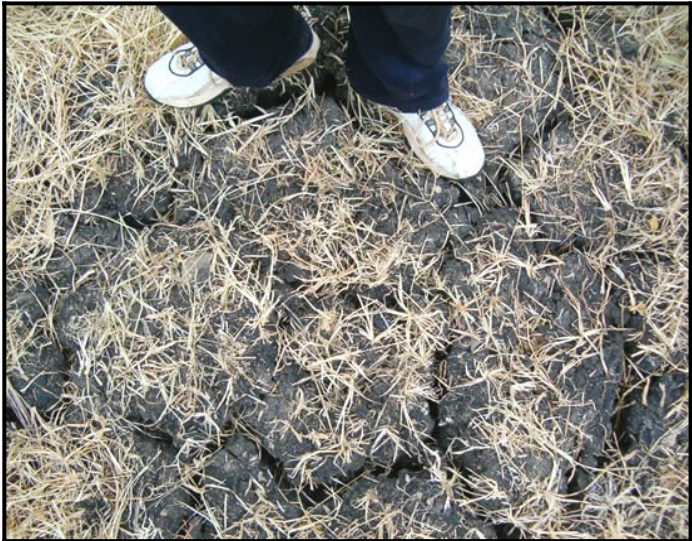
Figure III.2: Top view of the cracks in a Vertisol
