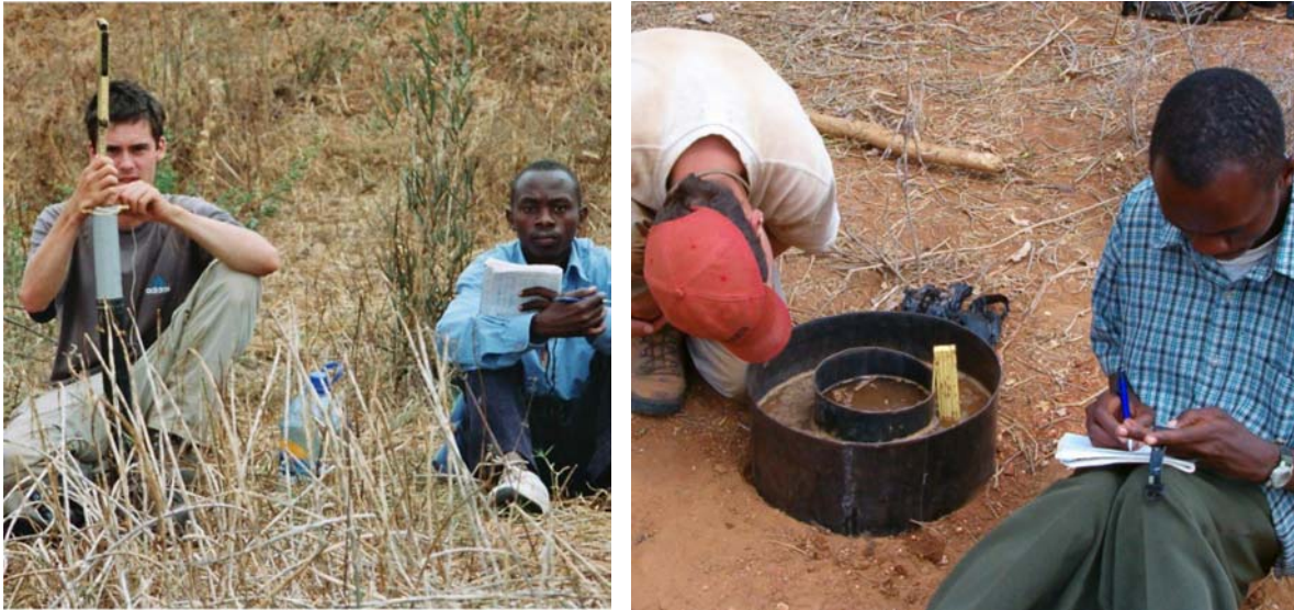
Figure 3.9: Methods for measuring the saturated hydraulic conductivity. The inversed auger hole method (left) and the double ring infiltrometer method (right).
